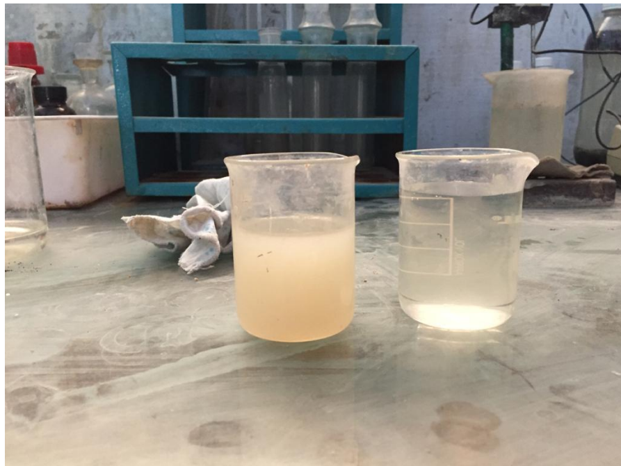
Fig. No. 4.3. WASTE WATER (LEFT) AND TREATED WATER(RIGHT)
